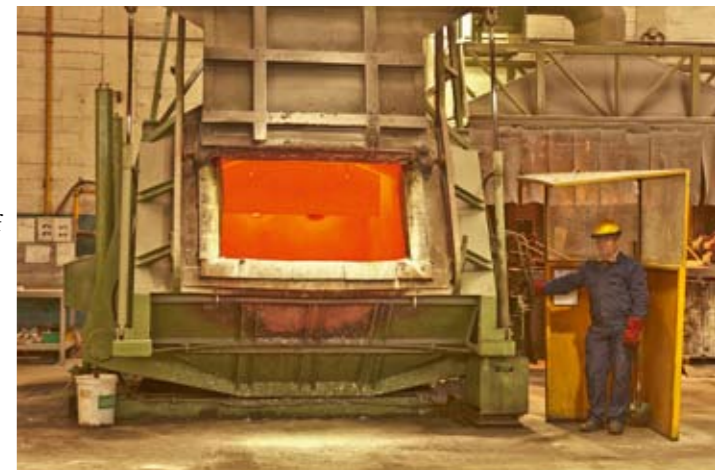
Above: vast supplies of 10kg aluminium ingots. Below: Ingots go into giant furnace at 800°C... and quickly change from solid to liquid (bottom pic)
