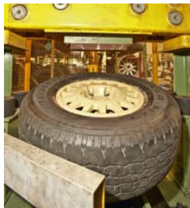
Above: 1550kg weight has just slammed down on this wheel, but you'd never know it!
